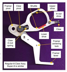
nut. Move the assembly to the right and lift it out, being careful to not damage the claw teeth or lose the two plastic shoes that fit on the shuttle and ride on the up-down cam. These might be black, white or red. If the Framer lever is the adapted type with a black plastic cap, this will just slide off.
