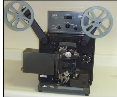
If the film has an optical sound track on it, turn the Sound Lamp switch to On. If the film is silent, you can turn the switch Off to extend the life of the sound lamp, and eliminate extraneous noises from being heard in the audio.
